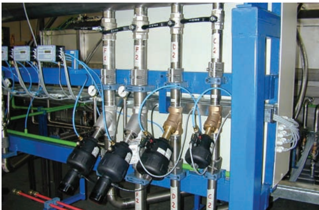
Time-saving installation due to the single bolt system; Integration of controls and instruments into an aluminium extrusion unit
