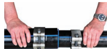
Push the tubes together as far as they will go.
